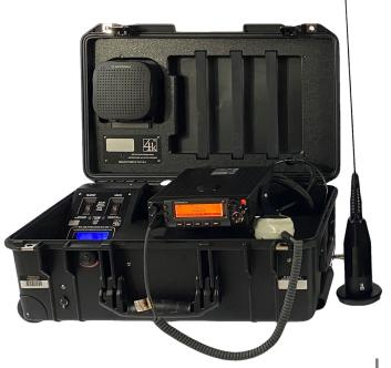
The Land Mobile Radio (LMR) Deployment Kit has an innovative lift, swivel and lock radio mount system to allow for the radio to be securely stored during transport. The Motorola Speaker is integrated into the lid to allow for loud and clear communications. The antenna and accessories are stored in the 4K Solutions® Pel-Pak™ kit bag which is provided and can be attached to the exteri-
