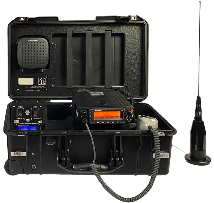
The **Land Mobile Radio (LMR) Deployment Kit** has an innovative lift, swivel and lock radio mount system to allow for the radio to be securely stored during transport. The Motorola Speaker is integrated into the lid to allow for loud and clear communications. The antenna and accessories are stored in the 4K Solutions® Pel-Pak™ kit bag which is provided and can be attached to the exterior lid of the kit.
