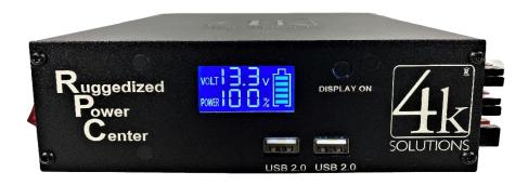
The **RPC** by 4K Solutions sets the standard for portable and rugged power. Using superior LiFePo4 battery chemistry, the RPC is lightweight, compact, and extremely powerful. The case is high-impact 6061 aluminum. The intelligent power meter is a sophisticated yet simple "fuel gauge", showing real time battery voltage and estimated percentage remaining. The **RPC** is chargeable from solar, a vehicle, or with the supplied AC charger, this machine is flexible and ready to work.
